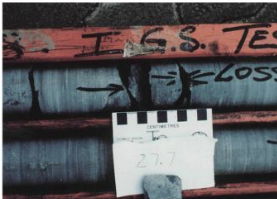
Figure 6-4 Photograph of a core sample that intersected the horizontal fracture on the Campus Test Site, displaying the fracture.
